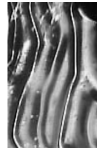
Fig. 3. The wide stripe-like domains in the R_I region. T = T_{NI}-2^{\circ}\text{C} , f = 1\text{kHz} , U_{th} = 36\text{V} , d = 12\mu\text{m} , crossed polarizers, magnification 100x.
